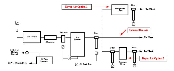
A complete compressor installation should include-
