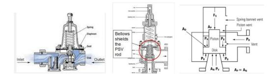
Direct operated PRV's of all three types are typically offered in sizes ½" through 2" with limited capacities. The directed operated PRV can be coupled with a larger valve with the pilot (a direct operated PRV) being the "brains" and the main valve being the "brawn".
