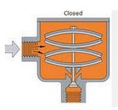
• I've included a cut away of an orifice trap to make the list but will again state I do not consider it to be a true steam trap since it fails the automatic part of sensing condensate and steam to provide proper operation. If you use this type of device,
