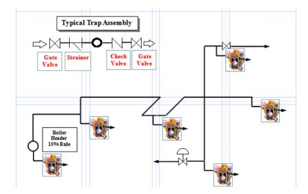
If wet steam continues to remain a problem, then adding a separator in the boiler plant or on selected primary and secondary lines is an option. Before adding a separator, trace all steam lines and make sure all steam drip traps are operating properly, then carefully review the piping to ensure that condensate is not being retained in pockets, sagging piping, or closed manual or automatic control valves. From Swagelok Energy Advisors, Inc.:
