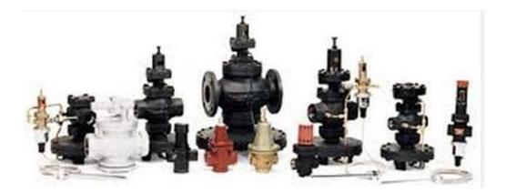
In this photo, the four smaller PRV's on the bottom are direct operated and by adapting them to a main valve, as shown by the larger valves on the top, can provide much higher capacities. Note that the same basic principle can be used to produce a direct operated temperature regulator using a bellows coupled to a thermal sensing system which allows a fluid to expand as it is heated, increasing internal forces on a valve shaft to open and close a valve based on temperature difference.
