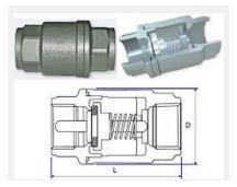
• <u>**Piston check valves**</u> use a spring loaded piston in a cylinder to provide both a positive shut off and also minimize slamming in the check valve when pressure pulses occur. They provide good service on the discharge side of steam traps and condensate pumps. Piston check valves should be installed in a horizontal orientation.
