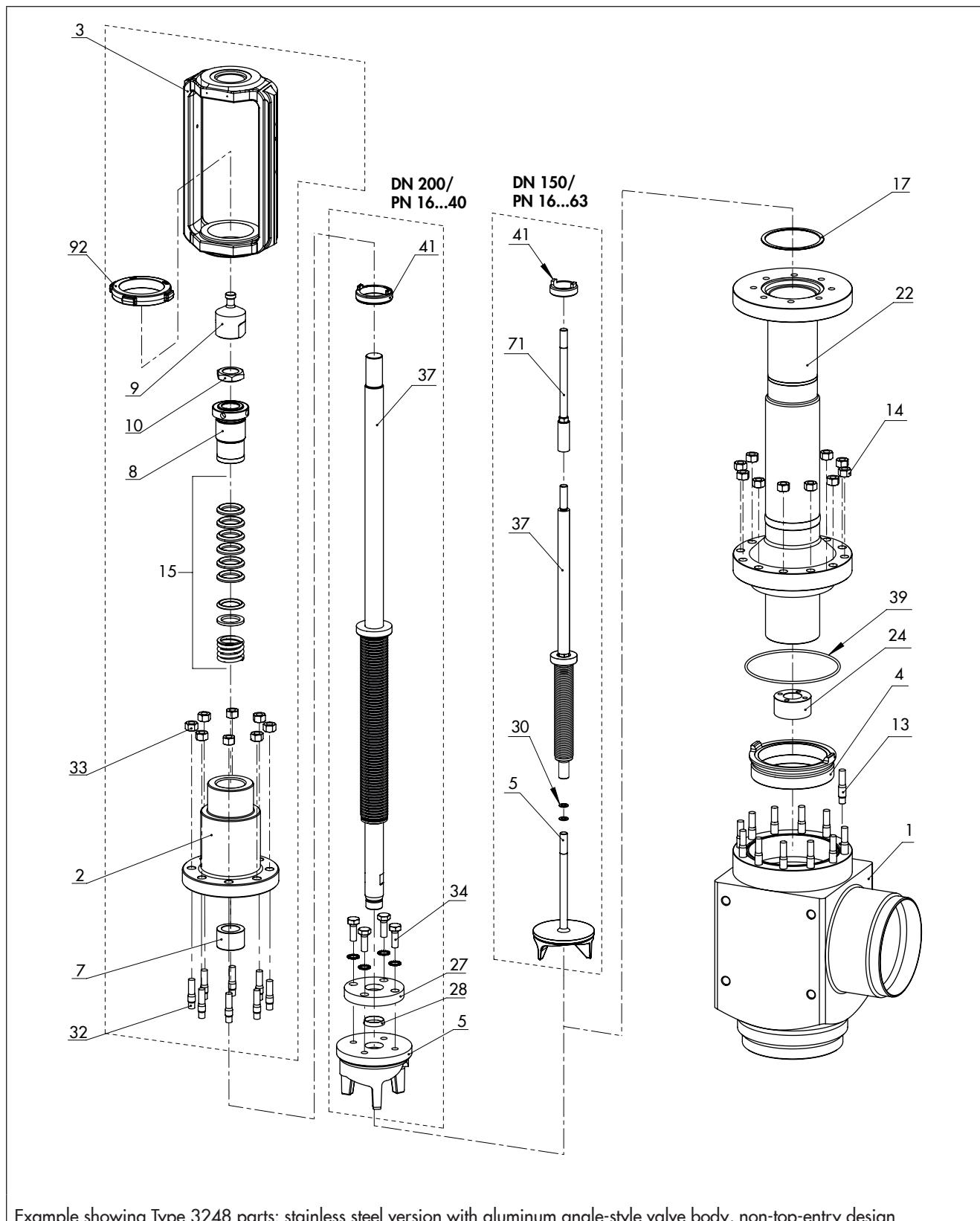
Example showing Type 3248 parts: stainless steel version with aluminum angle-style valve body, non-top-entry design
