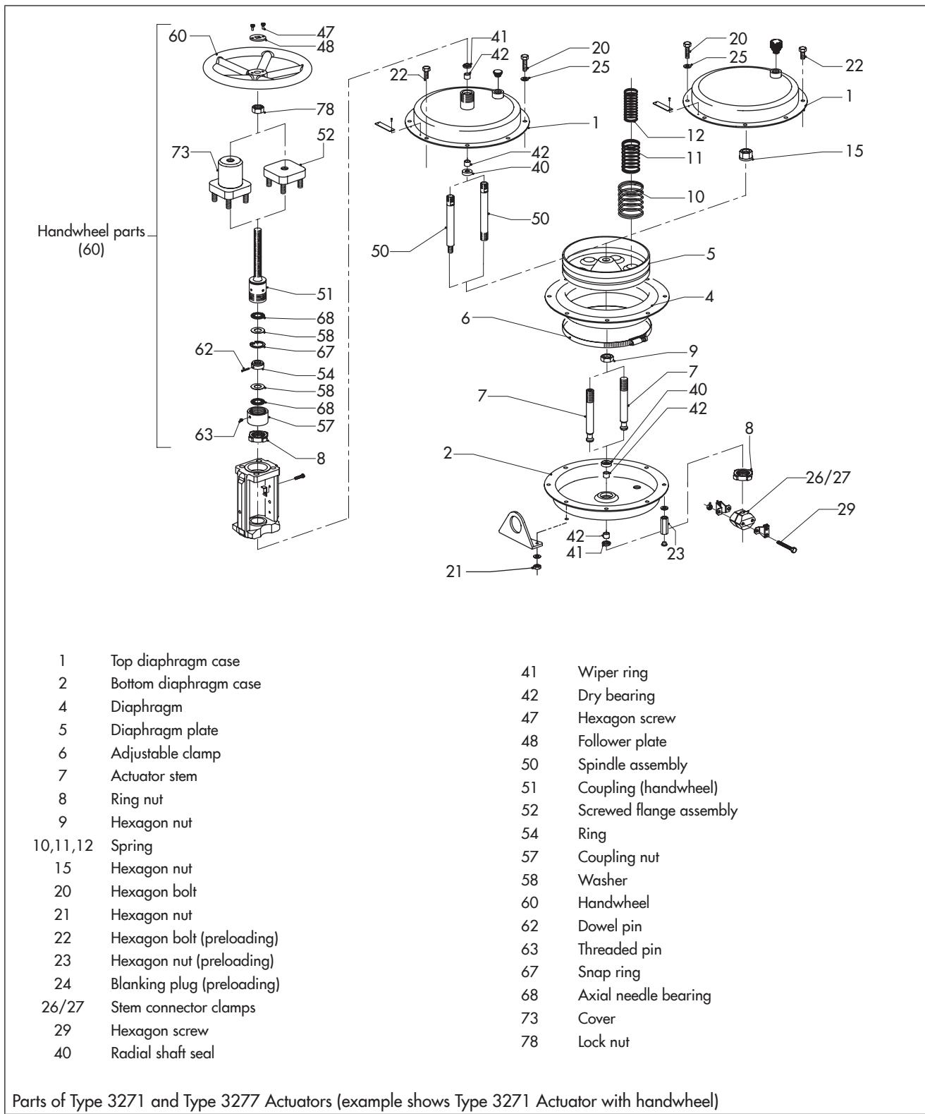
Parts of Type 3271 and Type 3277 Actuators (example shows Type 3271 Actuator with handwheel)
