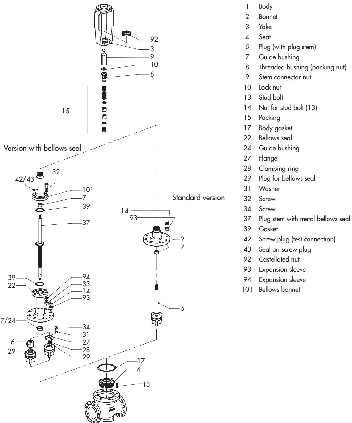
Parts for Series 250 Valves (example shows Type 3251)
