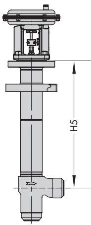
Angle valve with stainless steel body
