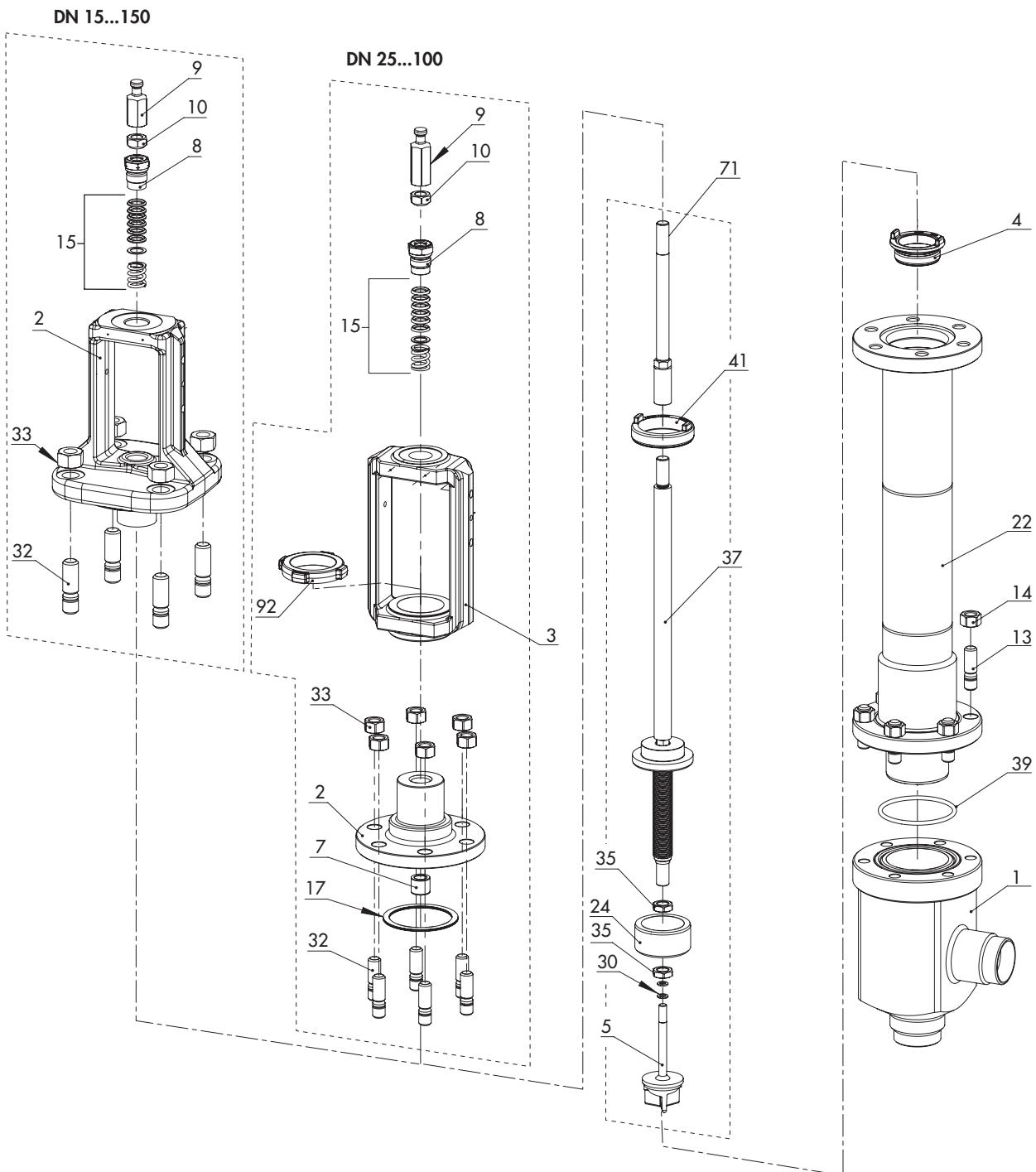
Example showing Type 3248 parts: stainless steel version with aluminum angle-style valve body, top-entry design
