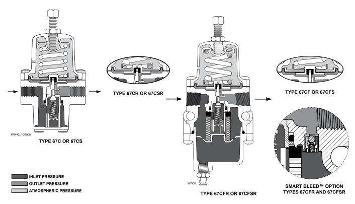
Figure 2. 67C Series Operational Schematics
