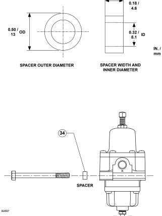
Figure 13. Spacer Diameter and Assembly (For Installing in an Existing Installation if the Mounting Bolts are Too Long)
