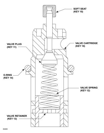
Figure 12. Valve Cartridge Assembly
