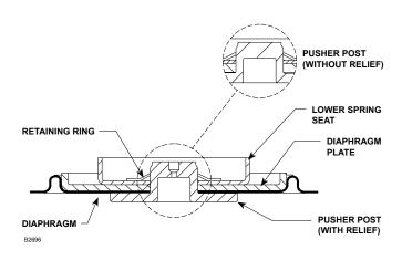
Figure 10. Diaphragm Assembly (key 16)
