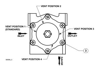
Figure 8. 67C Series Spring Case Vent Positions
