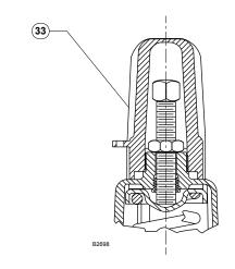
Figure 11. Optional Closing Cap (Only Available with the 1/4 in. / 6.4 mm Spring Case Vent)
