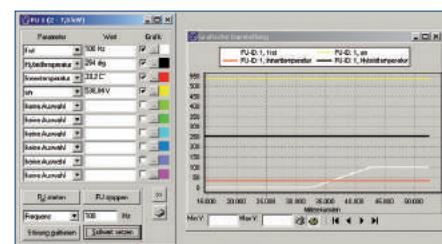
The software, together with a suitable interface converter, makes it possible to exchange data between a Becker frequency converter and a PC with Windows OS.
