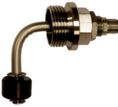
By default, the level transducer ST 682-0-5.1 is a normally closed contact that will switch (open) if the level falls (NC contact → magnet ring at the bottom). The float can be inverted by pulling out a locking ring. Now the contact will close when the level falls (NO contact → magnet ring at the top). The electrical connection is made via an M12 interface. The counterpart needed for the cable connection (an M12 bushing) is also included.
