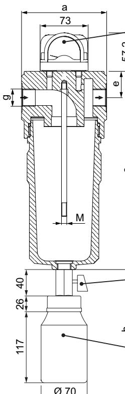
Incl. pressure differential gauge and integrated membrane for increased protection against contamination
