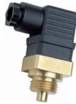
The bimetal thermostat built into the compact housing switches upon reaching the limit temperature. The contact is available as either NC or NO.
