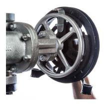
3. Fasten the adjustable clamp to valve hand wheel using the short L strap, a bolt, and a nut. Pass the bolt from step 1 through the short L strap and fasten with a nut.
