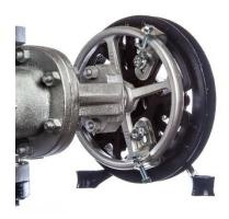
5. Center the chainwheel and tighten the nuts securely.
