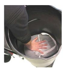
Push the elements down until all the trapped air has escaped out of the carbon elements.
