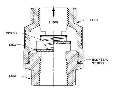
**WARNING**: If the system fluid is hazardous, take appropriate precautions. Make sure to bleed off pressure from the line before removing the valve. Hold the valve by the Hex end nearest to the mating pipe and loosen. Again, do not hold the valve by the opposite end, as this may loosen the valve body joint.
