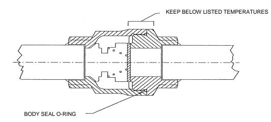
When welding the check valve into the line, avoid heating the marked body joint region above the temperatures listed below. Damage to the body seal (or optional soft seat) o-ring may result.
