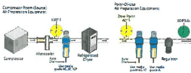
Any compressor with aftercooler, 2-stage coalescing, refrigerated dryer and carbon absorber. Air intended for use as industrial breathing air and decompression chambers. CAUTION: Always use high temperature synthetic lubricants and monitor (alarm for carbon monoxide concentration). This system will not eliminate toxic gases!
